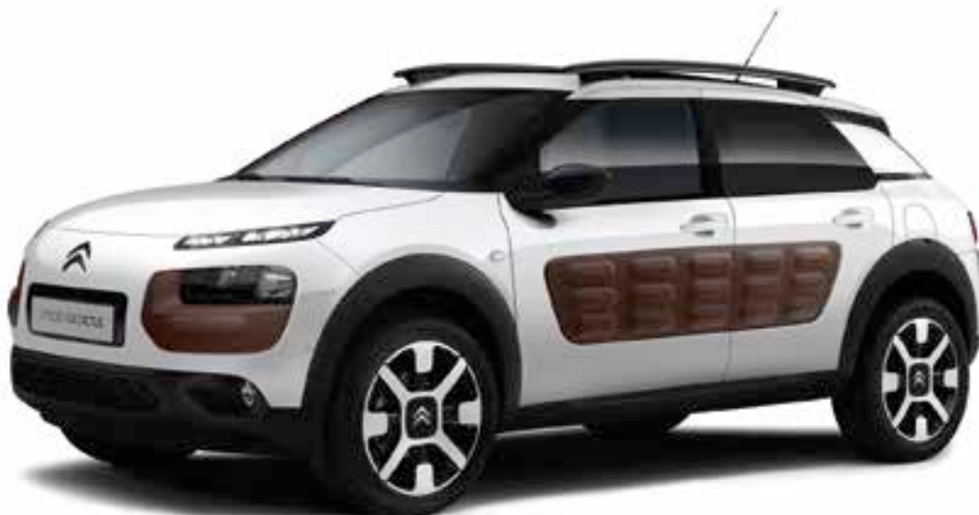
The Citroën C4 Cactus, with large, air-filled cushion bumpers in contrasting colors on the sides, front and rear
